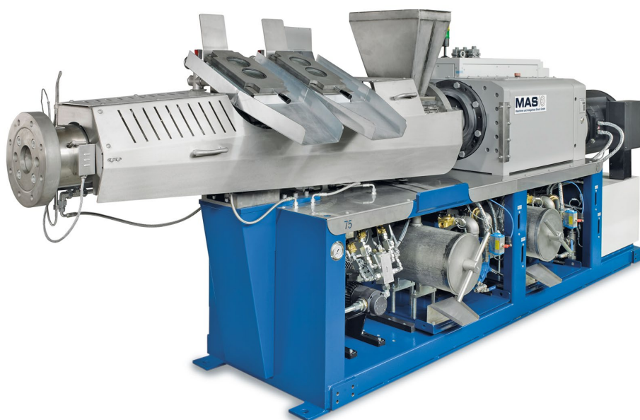
75-mm Twin screw PET lab-line by MAS
