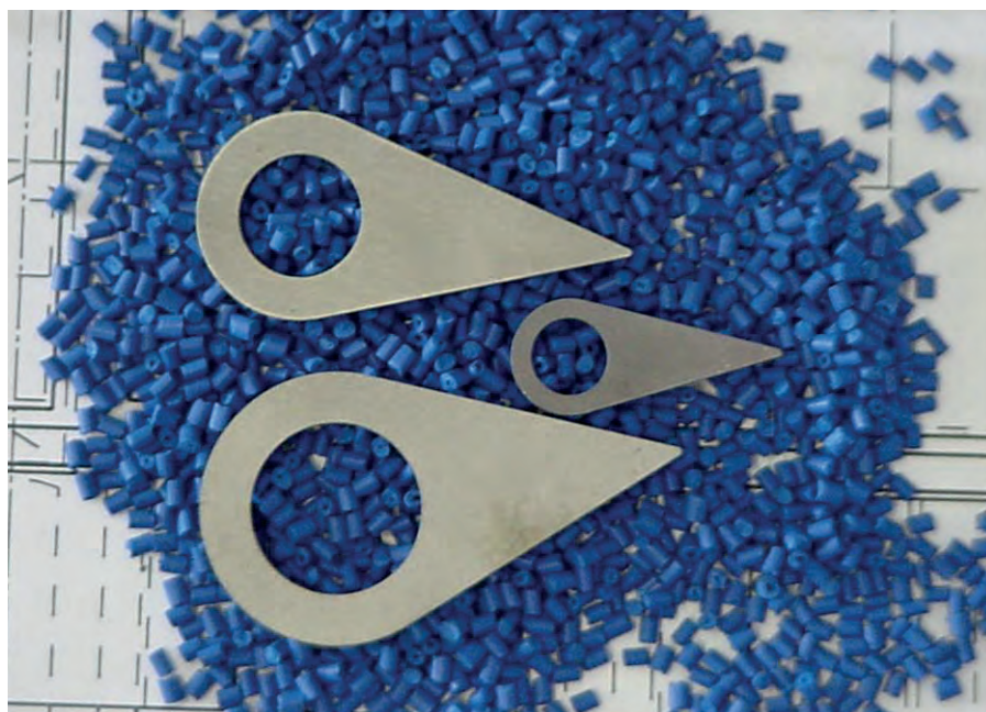
Only a few of the available lamellas for the KU7 feedblock.
